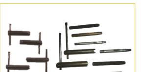
These bolt tightening keys are used to tighten nuts on conveyor belt fasteners for joining conveyor belts. These fasteners keys are manufactured from alloy steel & hardened. We manufacture two sizes of bolt tighten key for tighten nut for conveyor belt fastener No.1, 1½, No,2 & No2½, No3.
